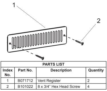
Two BRB Vent Register kits are needed for proper installation.
